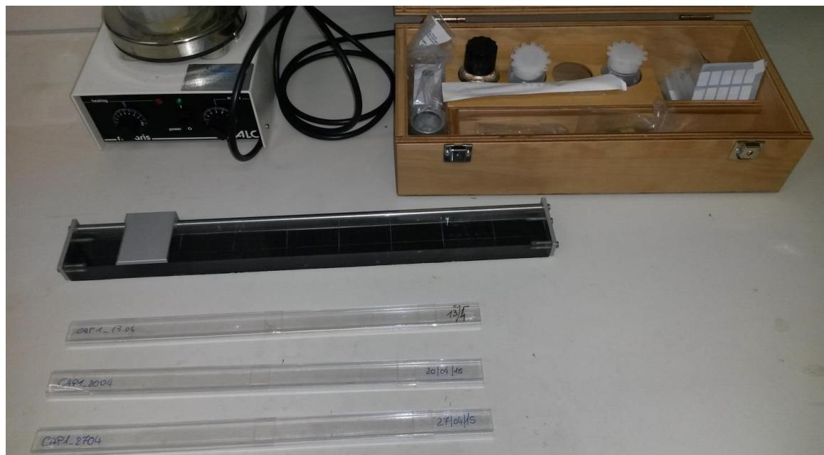
**5.** Preparation of slides: cutting of ribbons coming and collected weekly from the captaspore, fixing on a gel slide and subsequent observation to the optical microscope at 400 X
