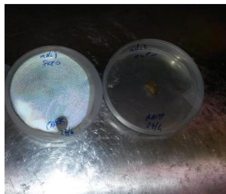
**1.-2. Photo of oomicities isolating method from apple bait:** The apple fragments were incubated on selective substrate Parp agar for the research of oomicities in surface water.
